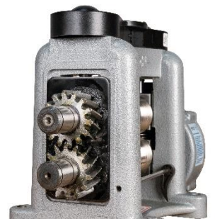
You can now grease the gears
