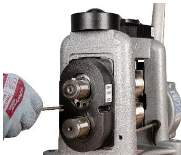
Remove 2 screws and cover
