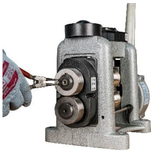
Remove black circlip (ring)
