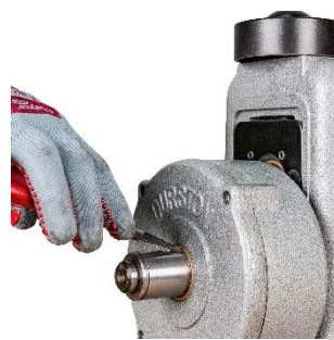
Remove 4 screws and remove circlip (ring)
