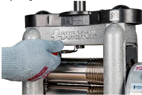
Remove black circlip (ring) on shaft
