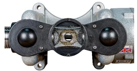
Move one of the gears, 1 tooth and replace handwheel assembly. Now roll material. Repeat this step (if necessary) until material comes out straight.
